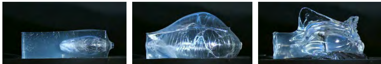
HyperSonic Bonded shows ultimate energy transfer on gel. 180 grain Core-Lokt Ultra Bonded bullet shot from 300 Win. Mag. shown.
