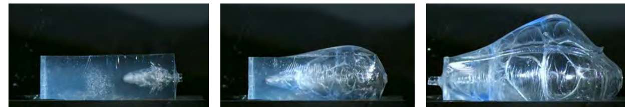
180 grain Core-Lokt Tipped bullet shot from 300 Win. Mag. shows extreme energy transfer and optimal penetration at 200 yards.
