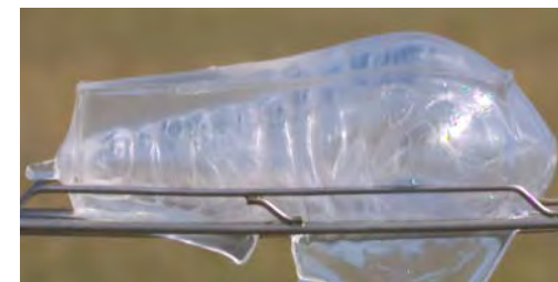
180 grain Premier Scirocco Bonded bullet shot from 300 Win. Mag. showing devastating expansion and energy transfer on gel.
