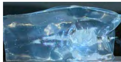
High speed videography time lapse of ballistic gel testing shows extreme energy transfer and wound channel expansion. Premier Long Range 172 grain .308 Win @ 200 yards shown.
