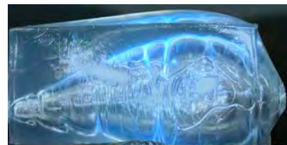
High speed videography time lapse of ballistic gel testing shows extreme energy transfer and wound channel expansion. Premier Long Range 172 grain .308 Win @ 200 yards shown.
